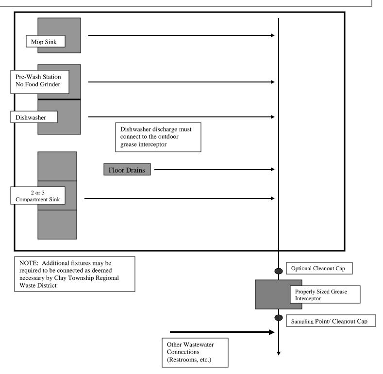
Grease Trap Installation Requirement:
