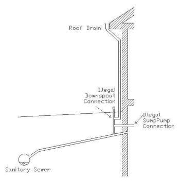
Downspouts illegally connected to the sanitary sewer system can be a huge source of clear water inflow. Roofs do not absorb water like soils and turfs. Therefore, rainwater that falls on a rooftop will leave the rooftop.
