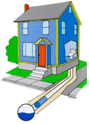
Defective laterals may also be a significant concern for the property owner. When water can infiltrate into the sanitary sewer system, soil particles can also migrate into the pipe and leave a subsurface void. These voids can cause sidewalks and patios to collapse. These voids also create sink holes that are a hazard. Some property owners believe they have a "perpetual sinkhole" where they continually add dirt, when in fact they have a defective lateral.
